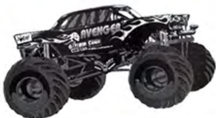
Name: Avenger Engine: 575 CI Big Block Chevy Transmission: Chevy Turbo 400 Make/Model: 1957 Chevy Bel-Air
