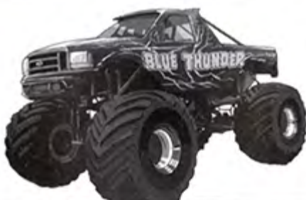
Name: Blue Thunder Engine: 540 CI Merlin Midget Transmission: COAN 2-Speed Make/Model: 2003 Ford Super Duty
