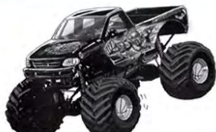
Name: Power Forward Engine: 540 Merlin Midget Transmission: COAN 2-Speed Make/Model: Ford F-150
