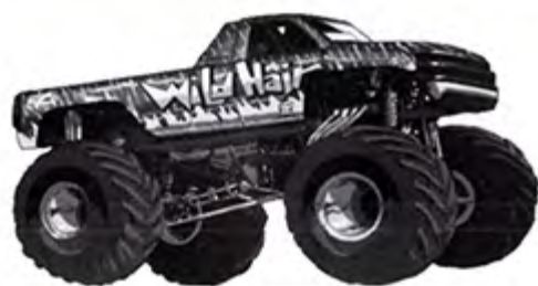
Name: Wild Hair Engine: 496 CI Lloyd Fischer Transmission: 400 Turbo Make/Model : 2002 Chevy Silverado
