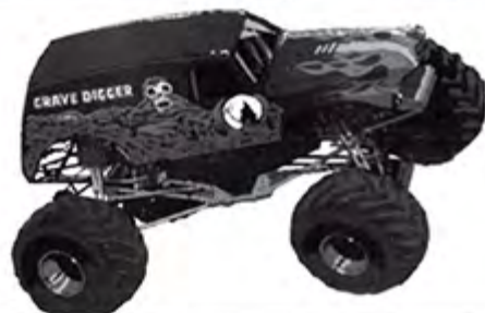
Name: Grave Digger Engine: 540 CI Merlin Midget Transmission: COAN 2-Speed Make/Model: 1950 Chevy
