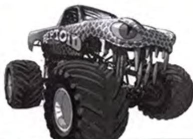
Name: Reptoid Engine: 540 Chevy Transmission: COAN 2-Speed Make/Model: Custom Reptile
