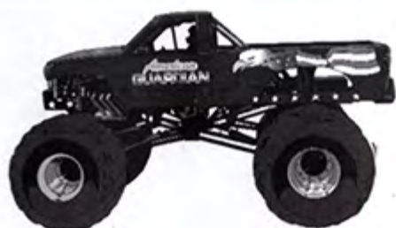
Name: American Guardian Engine: 520 Keith-Black Transmission: Chevy Turbo 400 Make/Model: 2002 Silverado
