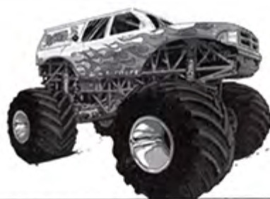
Name: Eradicator Engine: 428 Cobra Jet/Blown Transmission: COAN 2-Speed Make/Model: 2002 Dodge Durango SUV
