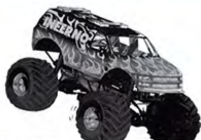
Name: Inferno Engine: 540 Merlin Midget Transmission: TH 400 COAN Make/Model: 1998 Chevy Astro Van
