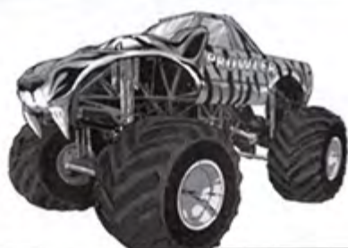
Name: Prowler Engine: 557 CI, All Aluminum, 1600 hp Transmission: COAN 2-Speed Make/Model: Custom Tiger
