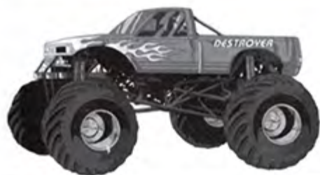
Name: Destroyer Engine: 540 Blown and Injected Transmission: 400 Turbo Make/Model: 2002 Chevy S10
