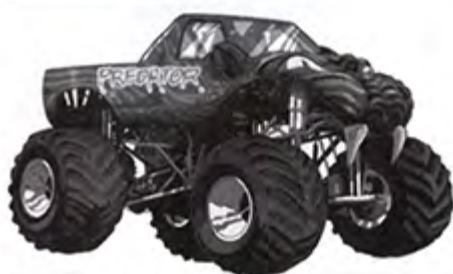
Name: Predator Engine: 557 CI, All Aluminum, 1600 hp Transmission: COAN 2-Speed Make/Model: Custom Panther
